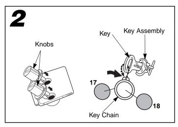
Snap the knobs into the knob plate.
